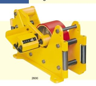
This is a heavy duty machine which measures the length of cable, wire, rope, hose, extrusions, or continuous strip from 6mm (0.24in) to 76mm (3.0in) diameter. Optionally this robust multi-purpose measuring machine is available with one side opening so avoiding the need to have access to the ends of the cable to start and finish measuring.
