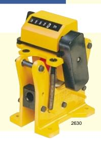
This robust machine measures the length of wire and other materials up to 15mm (0.59in) diameter. The 250mm circumference, precision ground measuring wheel runs in self lubricating bearings.
